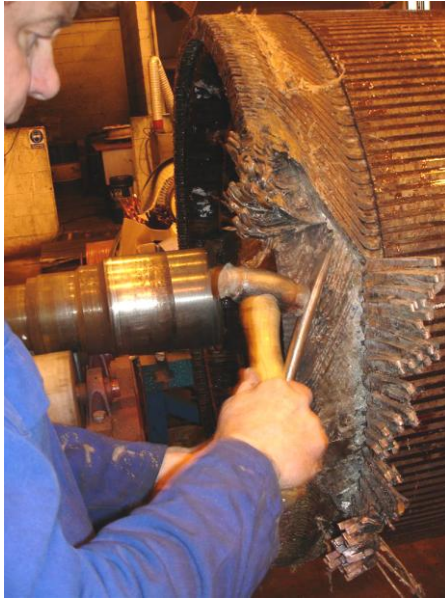
Damaged inner windings being knocked back. Photo by Mike Jacob.
