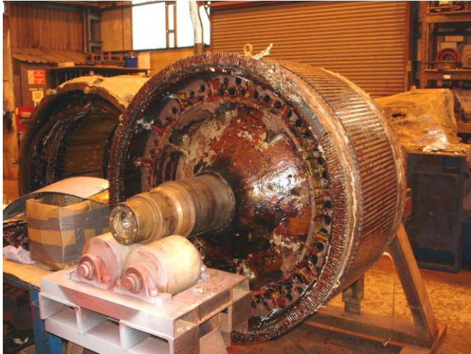
The damaged Armature, minus the Alternator Rotor, on Stands. Photo by Mike Jacob.
