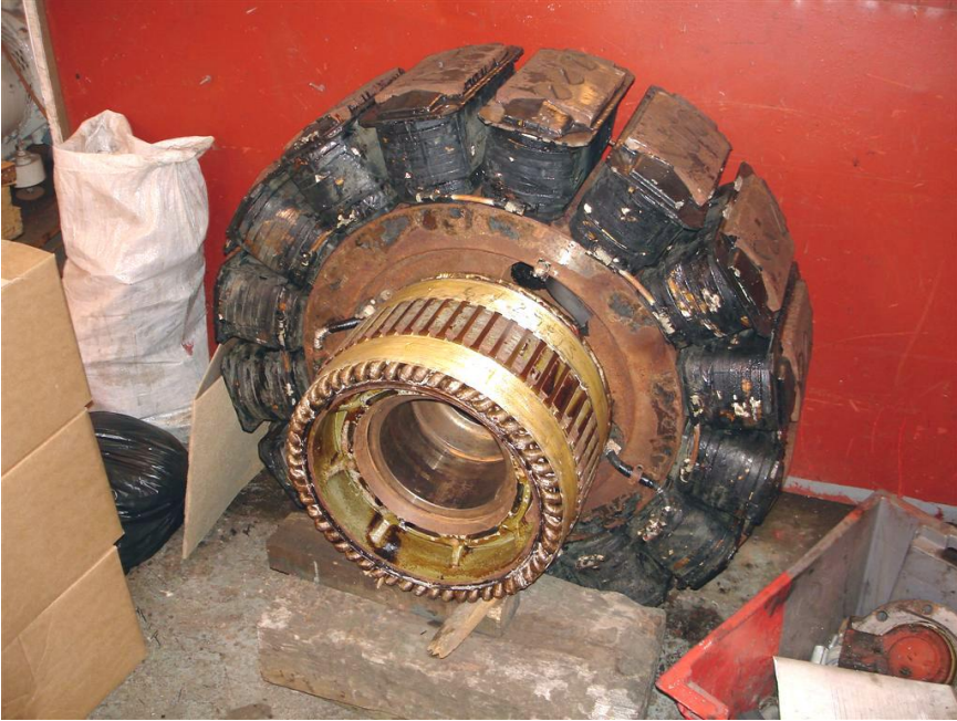
The Alternator Rotor separated from the main shaft. Photo by Mike Jacob.
