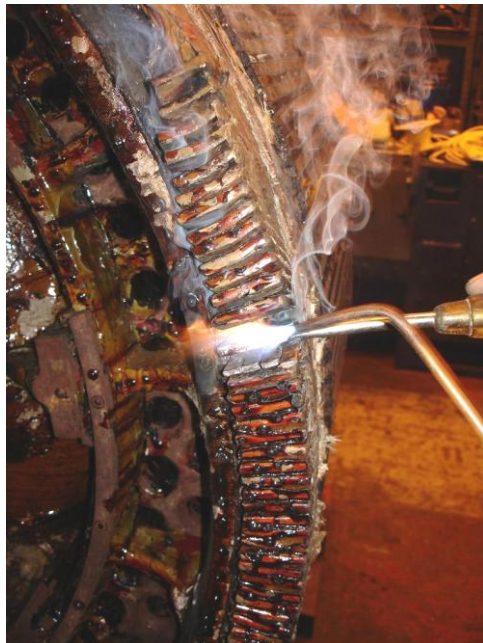
Melting off brazing connecting ends of windings. Photo by Mike Jacob.
