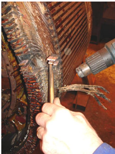
Top windings being prised out. Photo by Mike Jacob.
